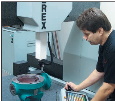
CMM evaluation of components are performed by PBV's Engineering and Testing Facility in Stafford, Texas.
